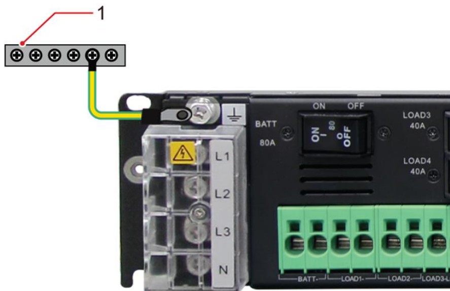
Figure 4-5 Connecting the ground cable
