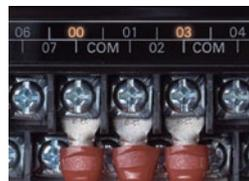
Reduce installation time and easily check wiring errors by LED indicators
