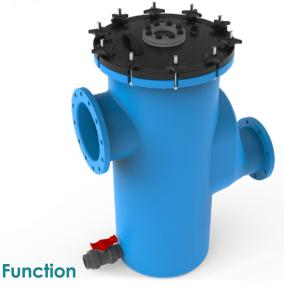
The strainer comes with a heavy-duty PVC basket that acts as a pre-filter for the protection of the pumps, meters, and valves. It is typically installed prior to the pump to catch large, solid impurities.
