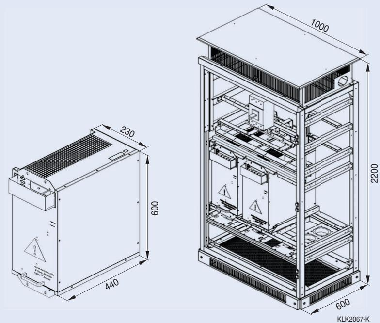
Drawings horizontal mounting variant (module 60 A/floor-mounted panel 300 A)
