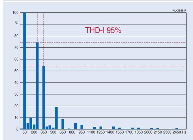
**Figure 3 Total harmonic current distortion with active filter**
