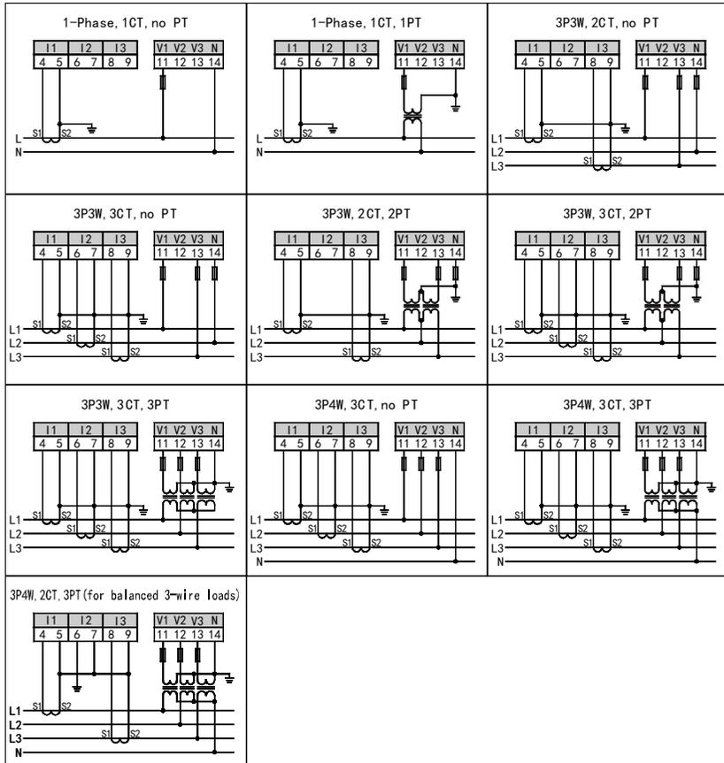
(a) Input voltage can not be higher than the rated input voltage (100V or 380V) of the product, or PT shall be considered to be used. For ease of maintenance, we recommend to use the terminal block.
