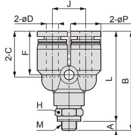
Appearance dimension for taper pipe thread (R)
