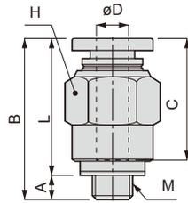
Appearance dimension for taper pipe thread (R)
