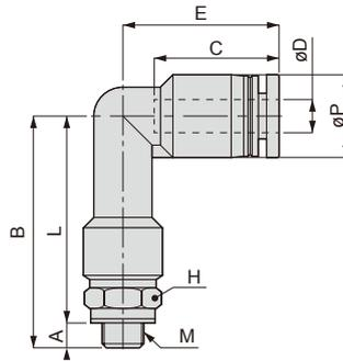
Appearance dimension for taper pipe thread (R)
