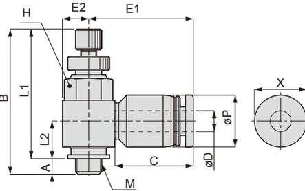
Appearance dimension for taper pipe thread (R)
