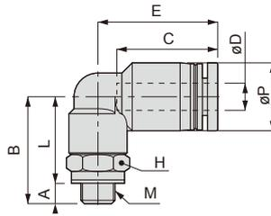
Appearance dimension for taper pipe thread (R)
