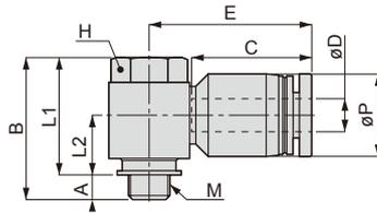
Appearance dimension for taper pipe thread (R)
