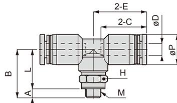
Appearance dimension for taper pipe thread (R)
