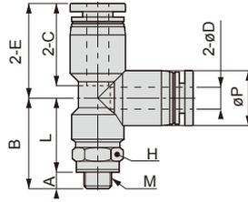
Appearance dimension for taper pipe thread (R)
