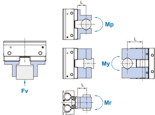
L: Distance to the point at which the load is applied (mm)
