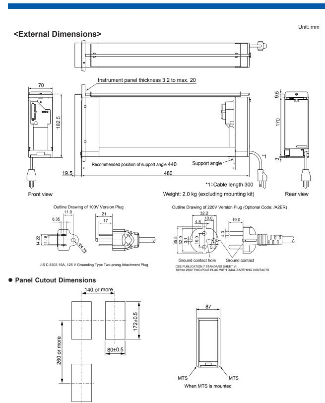
Note: If the YS series is mounted at an end in single mounting or side-by-side mounting, attach the separately sold mounting kit (MTS) to the housing.
