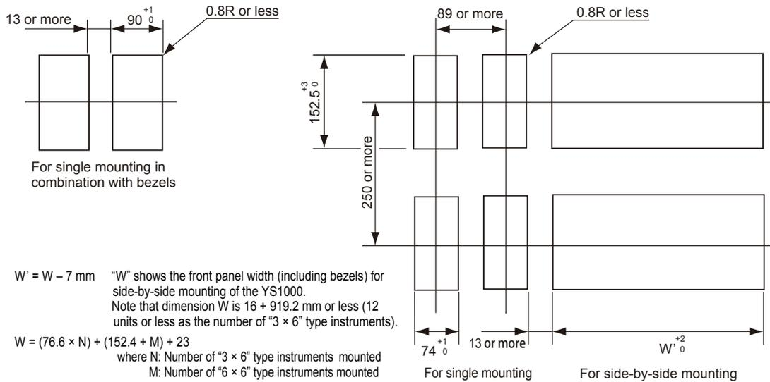
Note: If the YS series is mounted at an end in single mounting or side-by-side mounting, attach the separately sold mounting kit (RA001) to the housing.
