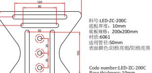
Code number:LED-ZC-200C Base thickness: 10mm Base size: 200x200mm Material:6061 Tube:50mm Color:Silver/Black
