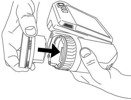
6. Rotate the inner ring of the lens 30° clockwise. The lens makes a click when it locks in place.
