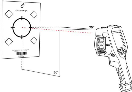
5. In the camera, align the thermal and visual images (indicated by the two squares in the image below), using the touchscreen arrows. The lens-camera combination is now calibrated.
