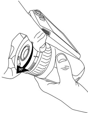
7. Make sure that the two index marks are aligned, indicating that the lens is locked in place.
