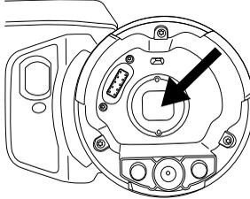
4. Make sure that the inner ring of the camera lens is fully in its open position.
