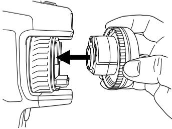
6. Rotate the inner ring of the lens 30° clockwise. The lens makes a click when it locks in place.
