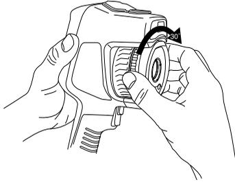
7. Make sure that the two index marks are aligned, indicating that the lens is locked in place.
