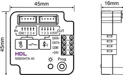
Figure 2. Dimensions-Front View
