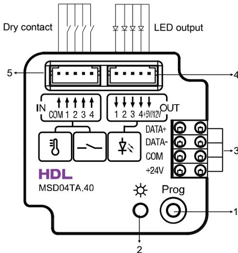
Figure 4. Wiring
