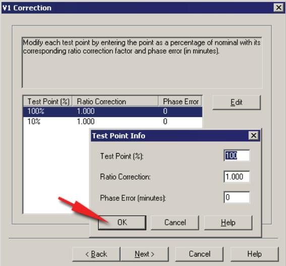
Modify each test point by entering the point as a percentage of nominal with its corresponding ratio correction factor and phase error (in minutes).
