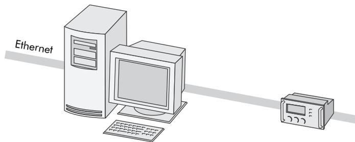
There are two Ethernet port ordering options available: a 10 Base-T port with an RJ45 modular connector or a 10 Base-FL port with two ST-type connectors. Both types of connectors plug into the Communications Module on the back of the meter. The meter supports a maximum of four simultaneous Ethernet connections.
