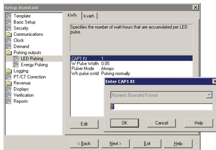
For **Digital Outputs**, select **Energy Pulsing** and select the tab of the energy pulsing value you want to configure. Edit the settings as desired.
