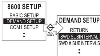
To view the Demand Setup menu via the meter's front panel, press and hold the **Alt/Enter** button. Press the **Up** or **Down** arrow buttons to highlight Demand Setup then press the **Alt/Enter** button.
