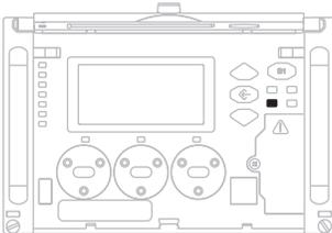
The recessed Master Reset button is located under the meter's front cover; it resets meter values. Use the Master Reset button to delete most accumulated values and all derived revenue measurements from the meter.
