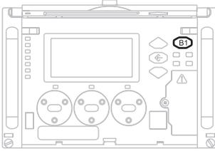
The recessed Demand Reset button resets the peak demand values logged in the meter. When the meter is in TEST mode, the Demand Reset button resets the test demand parameters.
