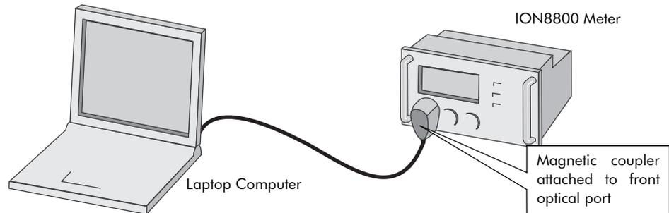
To enable communications from the optical port, configure the Comm 1 Communications module. The *Protocol*, the *Baud Rate* and *Unit ID* setup registers must properly match your system. When creating an ION site, ensure that RtsCts is disabled (set to No) in the COM1 serial site.
