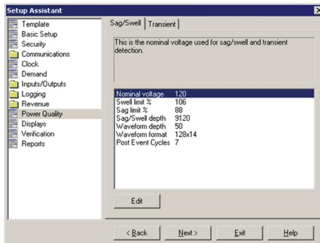
3. Select the **Sag/Swell** tab to set sag and swell limits, configure sag/swell waveform recorder settings and, most importantly, record your system's nominal voltage.
