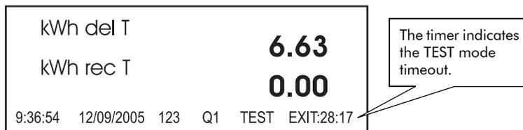
The time-out value resets to 30 minutes each time you press any front panel button. By default the TEST mode time-out value is 30 minutes.
