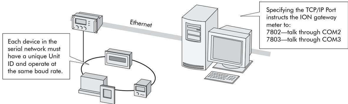
Once you have the chain of serial devices installed, use ION Setup or the meter's front panel to change the COM2 or COM3 Protocol setting to EtherGate. The transfer of data between protocols is then handled automatically.
