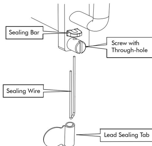
2. Twist the wire and crimp the lead sealing tab on to the wire.
