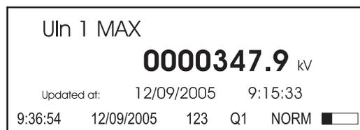
The front panel automatically scales the units for basic measurements (i.e. voltage, current and power parameters). For example, a measurement of 2,000 Watts is displayed as 2 kW. A measurement of 2,000,000 Watts is displayed as 2 MW. The meter makes these conversions using your PT and CT Ratios.
