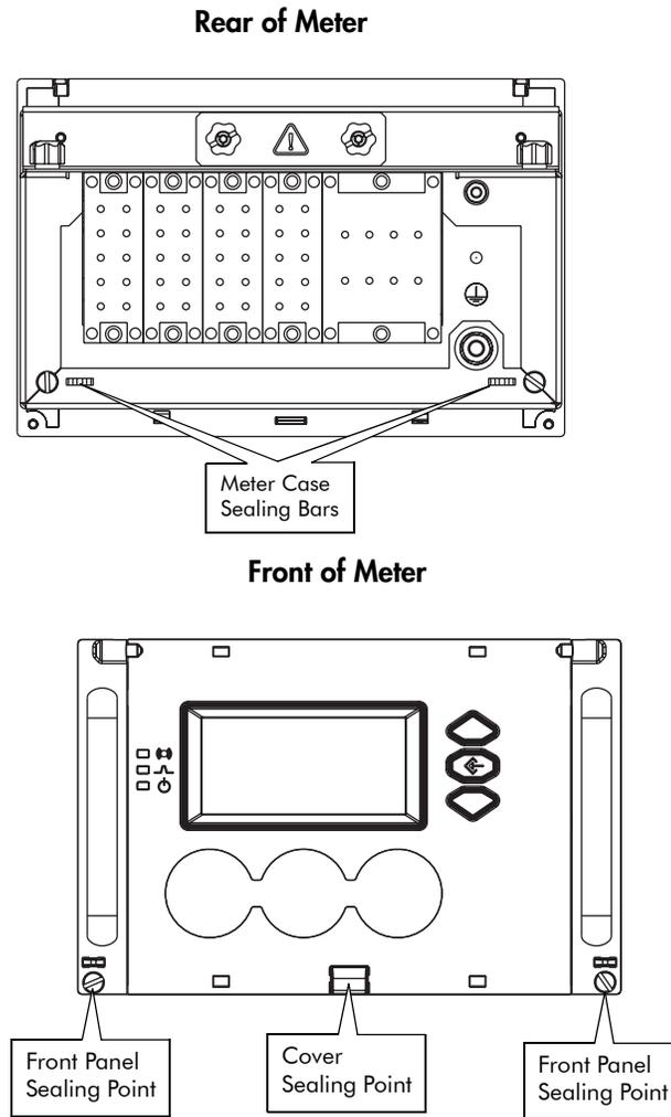
The meter incorporates sealing bars and chassis screws with through-holes, through which traditional lead/wire seals can be inserted. When utilized, these lead/wire seals effectively prevent unauthorized personnel from gaining access to meter internals or to buttons under the cover.
