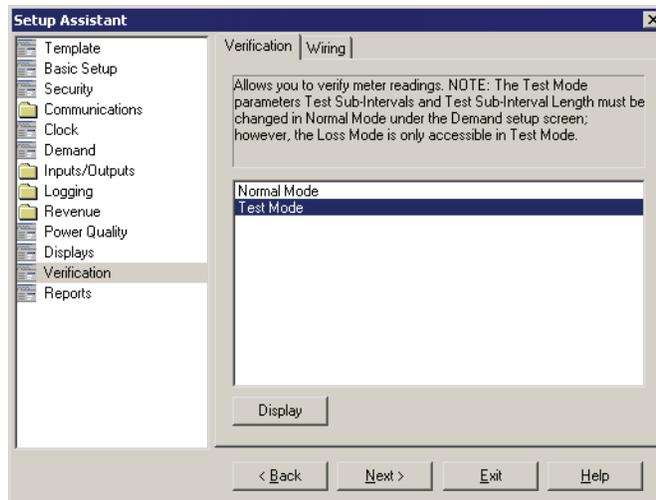
3. Select **TEST Mode** from the **Verification** tab. If meter security is enabled, you are prompted for password. A dialog box informs you the meter is in TEST mode.
