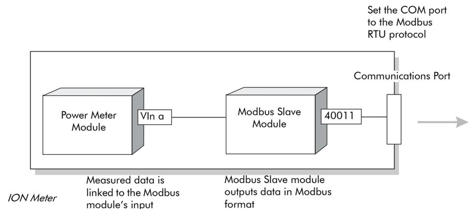
Since the data available through the Modbus Slave modules is in a specific format, knowledge of the Modbus protocol and an understanding of the settings used in the meter are required to interpret the data provided.
