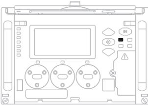
The recessed TEST Mode button is located under the meter's front cover; it places the meter into TEST mode. While in TEST mode, the meter ceases accumulation of billable quantities; energy and demand measurements are accumulated in TEST mode registers.
