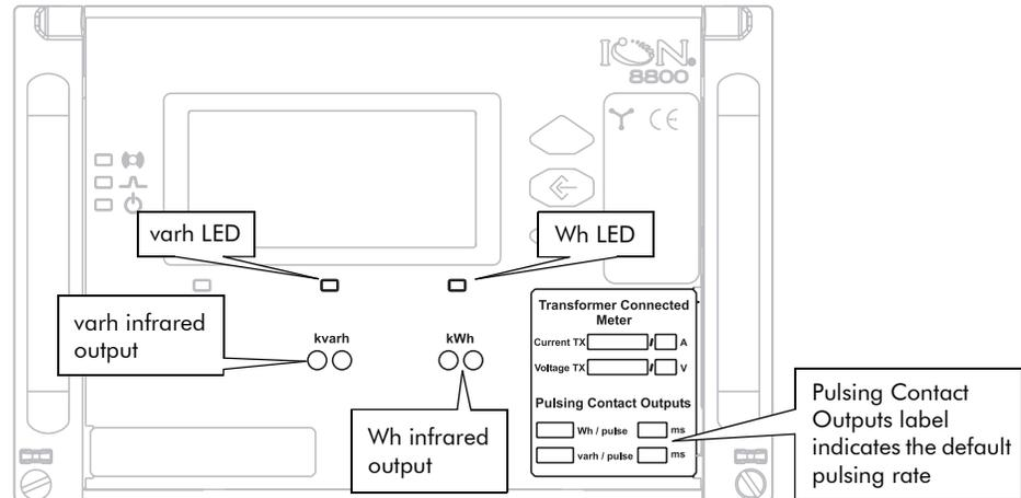
The energy pulsing LEDs provide an ideal interface for calibration checking instruments. The Pulsing Contact Outputs label (bottom right corner) indicates the factory-configured pulsing rate. (You can change the energy pulsing frequency with ION software.)
