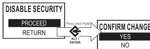
A message appears on screen notifying you of how to re-enable password security (refer to “Enabling the Password Security Check”, below). Your meter’s password is now disabled; changes to settings in the meter do not require a valid password.
