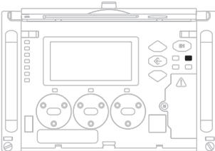
The recessed ALT Config button is located under the meter's front cover; press this button to access the Alternate Configuration menu.
