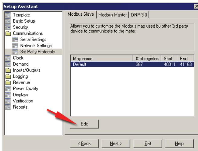
5. The default Modbus map editor appears, allowing you to edit, add, delete or set the name of Modbus Slave module registers.
