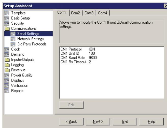
4. Click on the various tabs to configure the four serial ports (Com1, Com2, Com 3 and Com4). To change a setting, select the parameter and click **Edit**.
