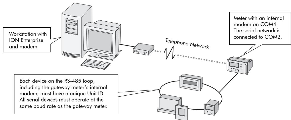
ModemGate connections do not connect a workstation with ION Enterprise (or other master device) to the gateway meter's COM2 or COM3 port, but rather the gateway meter's internal modem port (COM4).
