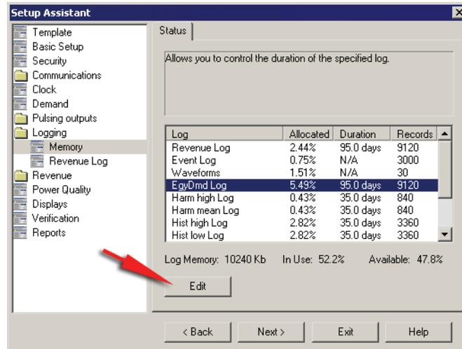
4. Select the Log you want to configure and click **Edit**. You can change both the Log Duration (days) and the Log Size (records). Notice how changing these parameters affects the meter memory allocated to that log.
