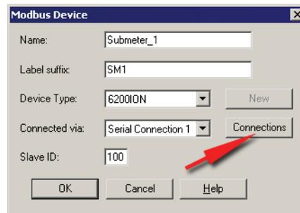
9. Click **Connections** to edit the serial connection used by the Modbus Master to connect to this Slave device. Note that the ION8800 meter currently does not support downstream TCP connections for Modbus mastering.
