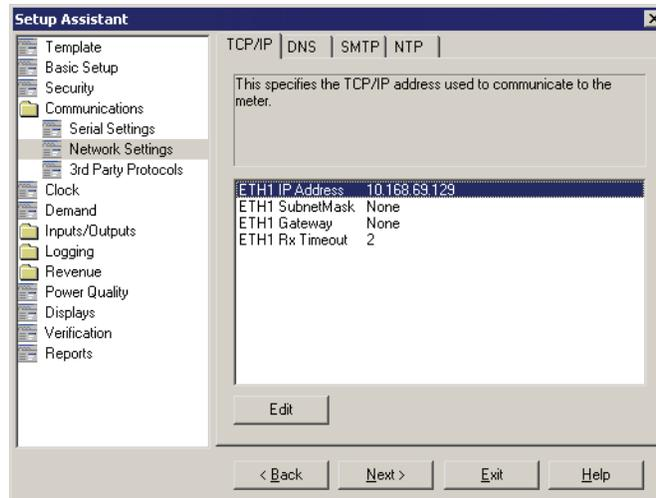
4. Click on the various tabs to configure the meter's TCP/IP, DNS, NTP and SMTP settings. To change a setting, select the parameter and click **Edit**.
