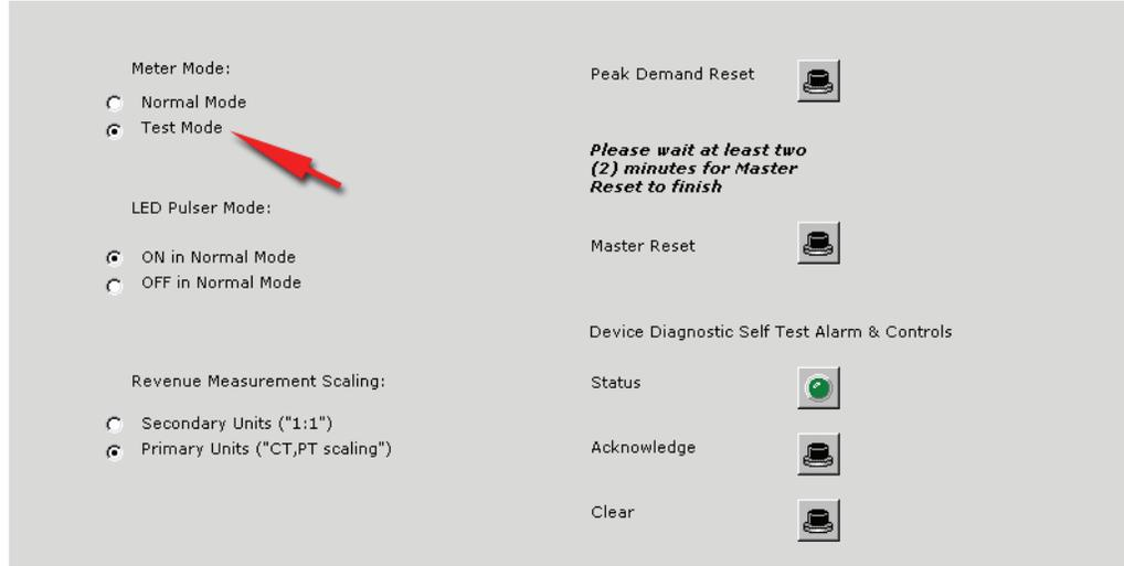
Use this screen to reset the registers that accumulate real-time data.
