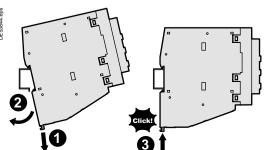
Installing the SC150 module on DIN rail
