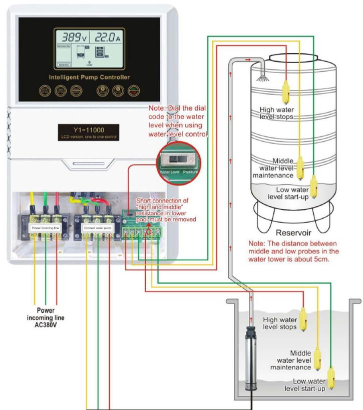
**Note: Avoid Signal Line Short Circuits: Ensure no entanglement with power or pump lines, and steer clear of areas with strong interference from electrical appliances like transformers or signal towers.**
