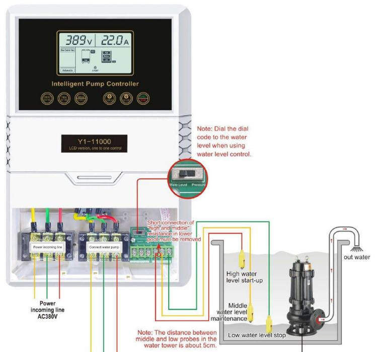
**Schematic diagram of wiring, using a pressure switch for constant water pressure supply.**
