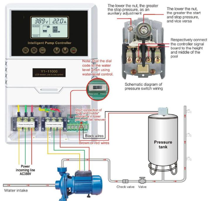
**Note: Avoid Signal Line Short Circuits: Ensure no entanglement with power or pump lines, and steer clear of areas with strong interference from electrical appliances like transformers or signal towers.**
