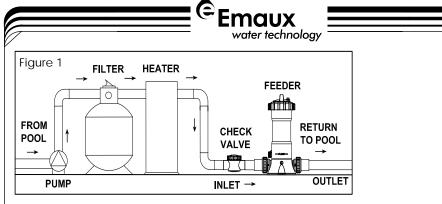
At the inlet pipe to the feeder, a positive seal corrosion-resistant check valve should be installed to reduce backflow of chlorine gas when the system is turned off. It is recommended that if the feeder is installed below the waterline, a check valve is needed to prevent water backflow when opening the unit.
