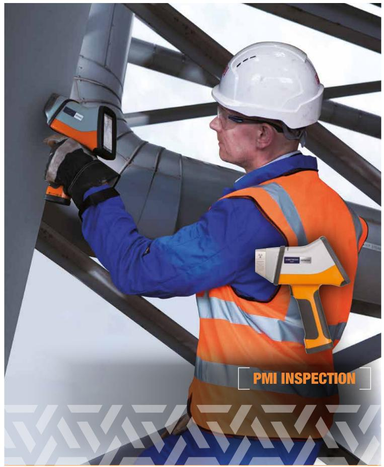
The X-MET8000 is a handheld X-ray fluorescence (XRF) analyzer that delivers ultimate on-site alloy analysis for safety critical applications. material inside bends and corners. And thanks to our unique HERO™ (heat resistant) window, With X-MET8000 you can minimise laboratory testing and reduce costs whilst ensuring safety
