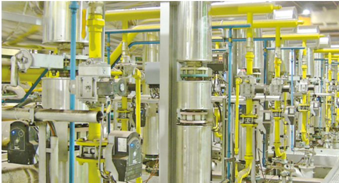
Walking beam furnace with overhead firing
