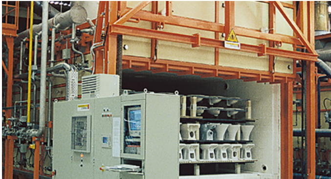
Intermittent shuttle kiln in the ceramics industry
