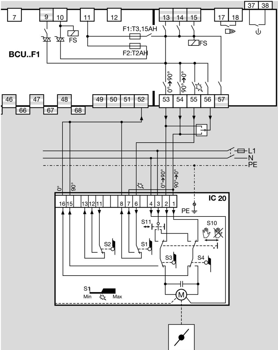
**IC 20..E connected to BCU..F1**
