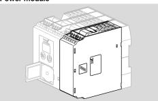
Suitable for control units BCU 500 or FCU 500. With relay contacts for the fail-safe outputs, e.g. for fan, butterfly valve and valves. To replace a power module with the same identification number if fault 36 is displayed.
