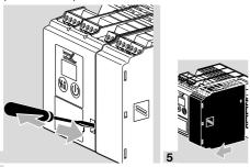
6 Having removed the power module, replace the parameter chip card if required.
